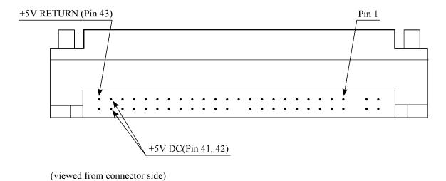
Figure 3.8 Power supply connector pins (CN1)
